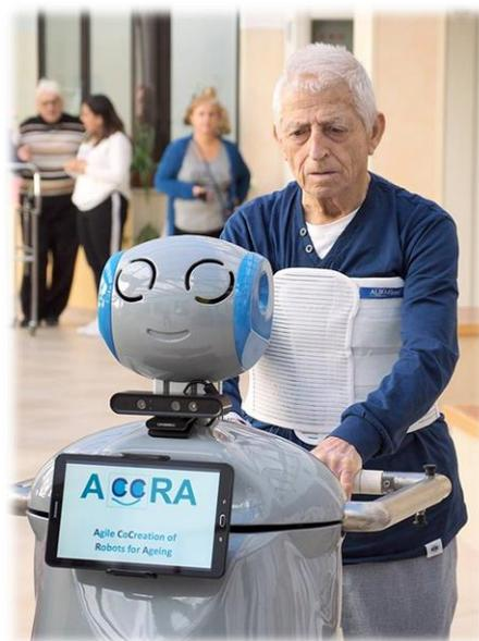
Astro is a robot for mobility assistance and rehabilitation, used in hospitals or retirement homes. This robot was developed by Santa Anna University in Italy.
